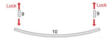
Lock [9] into pillslots on concave side of header support
